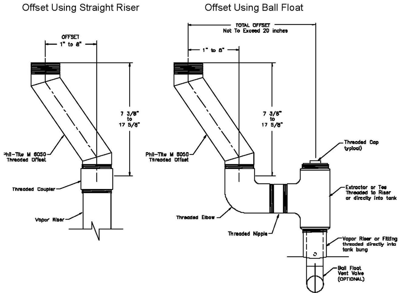
**Note:** This figure represents one instance where a vapor recovery riser has been offset in order to construct a two-point Phase I vapor recovery system. The above figure illustrates an offset using a 90-degree elbow. However, in some instances, elbows less than 90 degrees may be used. All fittings and pipe nipples shall be 4-inch diameter similar to those of the spill container and rotatable Phase I adaptors in order to reduce back pressure during a gasoline delivery.
