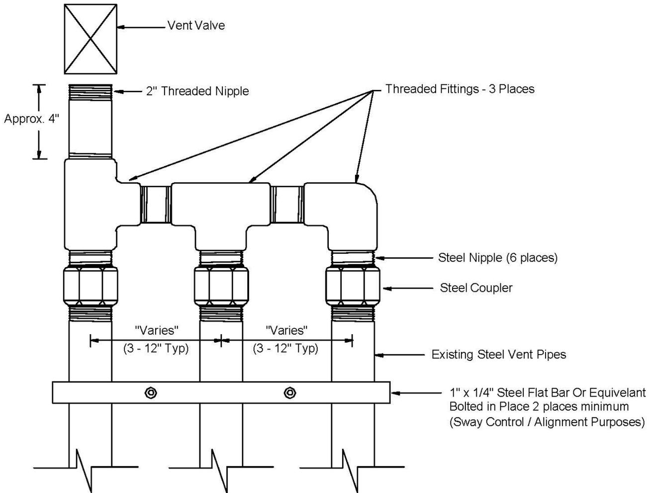
**Note:** This shows one typical configuration; other manifold configurations may be used. For example, a tee may be located in a different position, or fewer pipes may be connected, or more than one P/V valve may be installed on the manifold.
