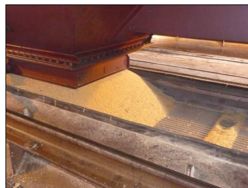
Figure 1. Railcar receiving choke flow
