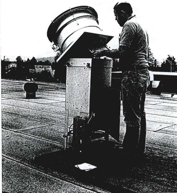
A white quartz filter is placed on the PM-10 sampler in order to capture the fine particulate matter for later laboratory analyses.
