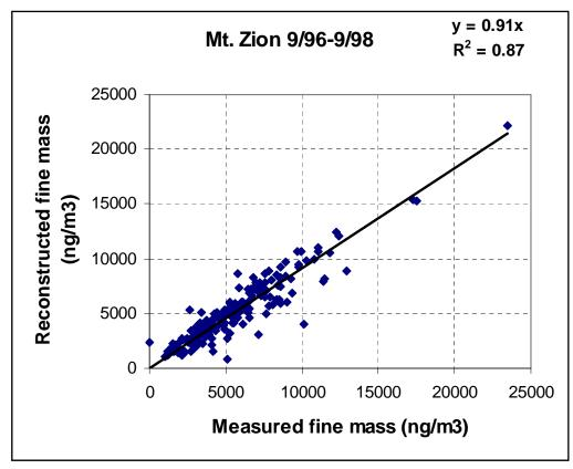
Figure 2-6. Measured versus reconstructed mass, Wishram and Mt. Zion 9/96-9/98.
