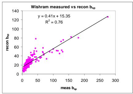
Figure 2-13 Measured versus reconstructed particle light scattering, Wishram – 9/96-9/98.
