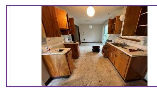
02- Octagon Pattern Sheet Vinyl Flooring and Mastic in the Kitchen in good condition. Mastic associated with Sheet Vinyl Flooring is non detect for asbestos.
