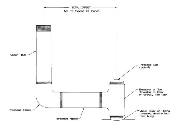
Note: This Figure represents one instance where a vapor recovery riser has been offset in order to construct a two-point Phase I vapor recovery system. The above Figure illustrates an offset using a 90-degree elbow. However, in some instances, elbows less than 90 degrees may be used. All fittings and pipe nipples shall be 4-inch diameter similar to those of the spill container and rotatable Phase I adaptors in order to reduce back pressure during a gasoline delivery.
