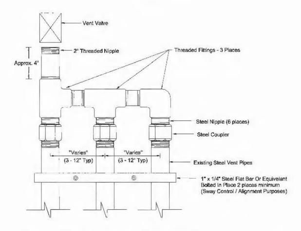
Note: This shows only one typical configuration; other manifold configurations may be used. For example, a tee may be located in a different position, or fewer vent pipes may be connected, or more than one P/V valve may be installed on the manifold.
